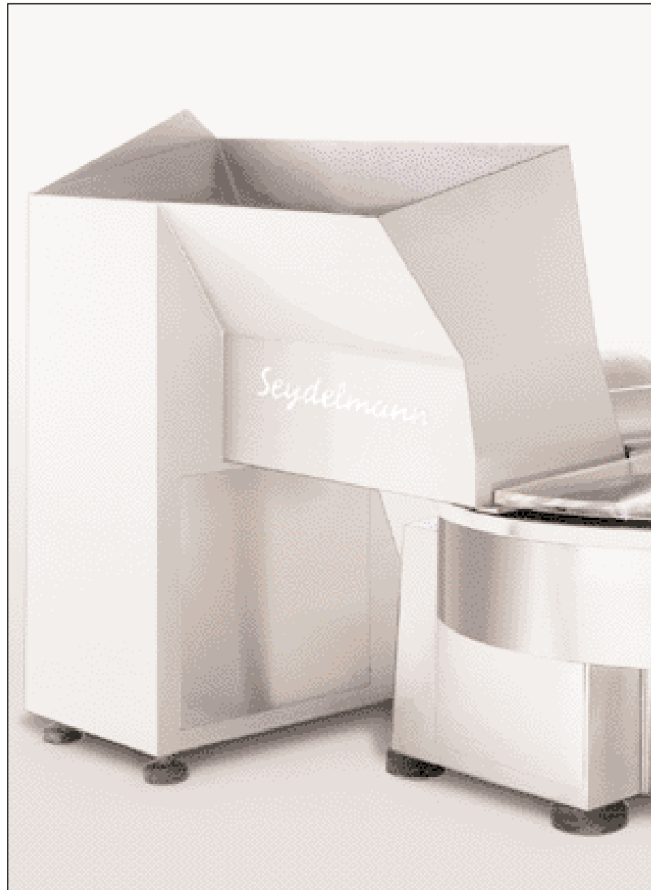
Loading via screw conveyor with hydraulic sliding valve
