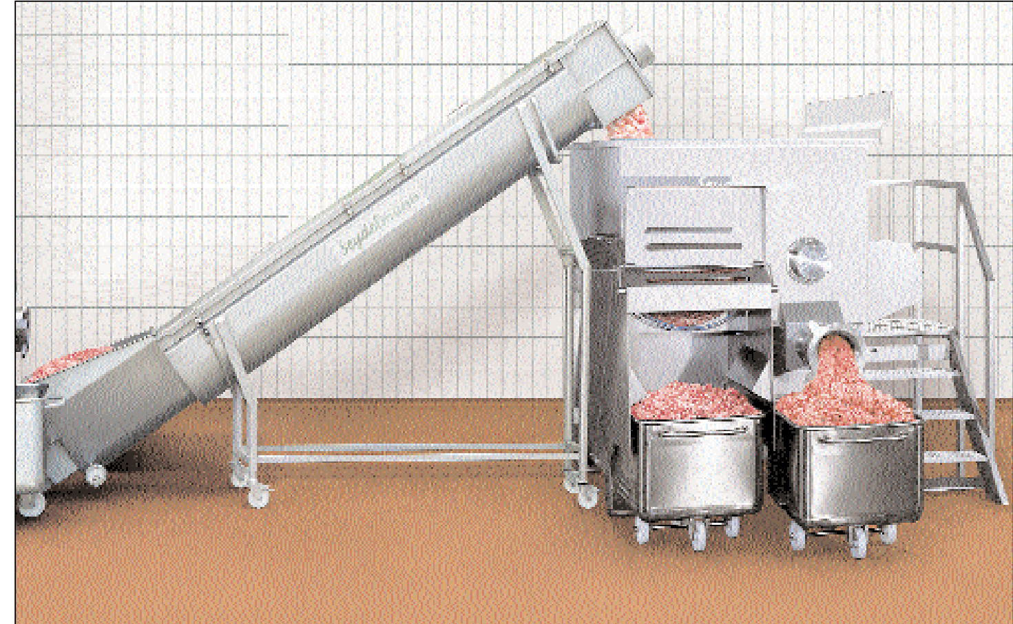
Mixer-Grinder PG 160 with movable screw conveyor (unloading as a standard on the left hand side, on request on the right hand side)
